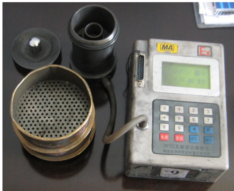
Figure 4. Chinese Desorbometer with sieve, internal container to hold cuttings and external part to provide dead volume and electronics to measure change in pressure within the container over a period.
