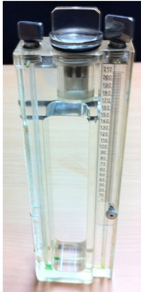
Figure 3. Polish Desorbometer to measure gas release from sieved sample (between sizes) of known volume versus a manometer.
